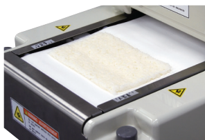
1. It spreads sushi rice onto the forming sheet
